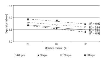
FIGURE 1. The expansion ratio of pasta processed with different moisture content of dough from a flour type 450 and 2% of salt under various extrusion screw speed.
