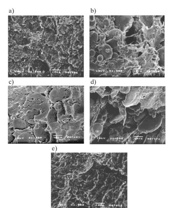
FIGURE 3. Cross-section of precooked pasta processed under different conditions at x1500 magnification: a) flour type 500, 28% m.c., 60 rpm, b) flour type 500, 30% m.c., 80 rpm, c) flour type 500, 32% m.c., 100 rpm, d) flour type 450, 30% m.c., 80 rpm, e) flour type 550, 30% m.c., 80 rpm.
